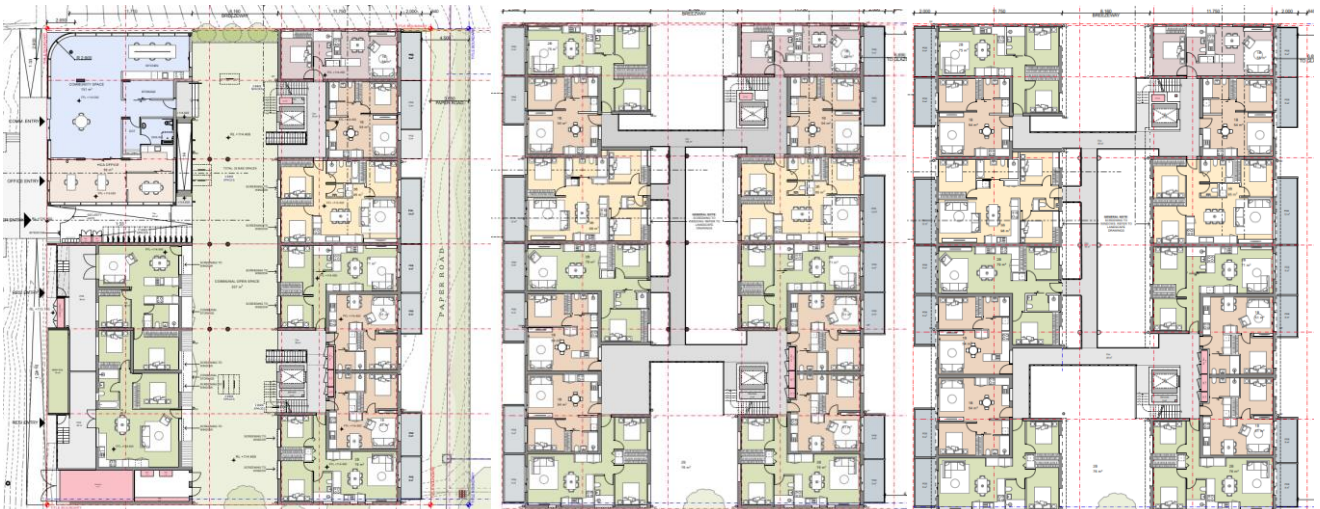
Excerpt from Freadman White Architectural Plans (Ground, Level 1, Level 2) showing floorplate efficiency and access to light, ventilation and outlook.
